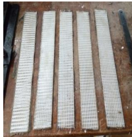
Fig. 5. Casted A-R glass fiber mesh GFRP
