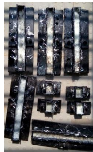
Fig. 6. Casted chopped E glass fiber GFRP
