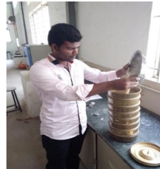
Figure 2a Sieve Analysis of FA
