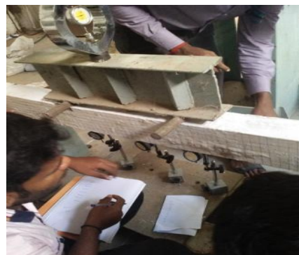
Figure 5 Bending test on Beam
