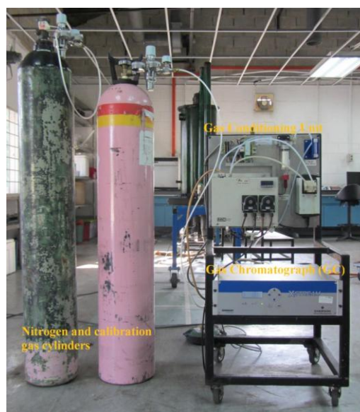
Figure 3. Picture of online gas sampling and gas analyzer unit with calibration gas cylinders
