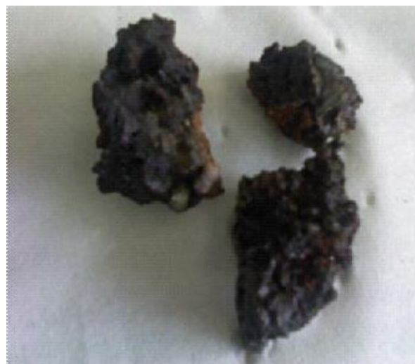
Figure 13. Picture of a sample of clinker or ash fusion produced at the grate
