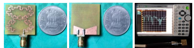
(a) top view (b) bottom view (c) measured S11
