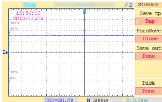
Fig 14. Waveform for filtered rectified dc output voltage
