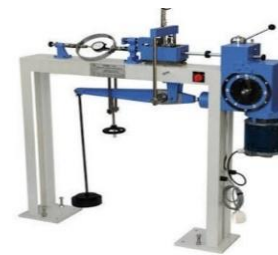
Fig3: Direct shear test apparatus
