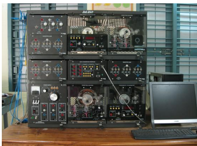
Figure 3. Induction motor built with LVDAM-EMS interfaced system
