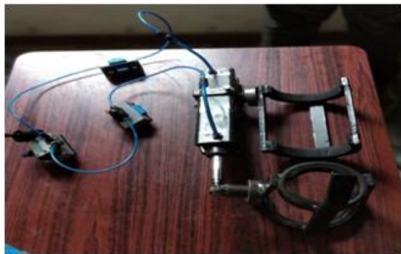
Figure 3: Fabricated model of Pneumatic Exoskeleton Arm
