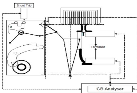
Figure 2: Schematic Representation of the CB Analyzer Test Setup
