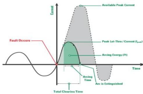
Figure 1: Normal Short Circuit and Current Limiting
