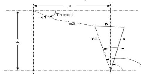
Figure 3: Representation of the contact system as a 4-bar linkage
