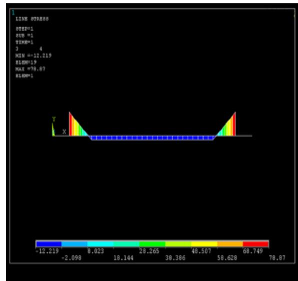
Figure 9: Maximum stress developed along the length of the Pin
