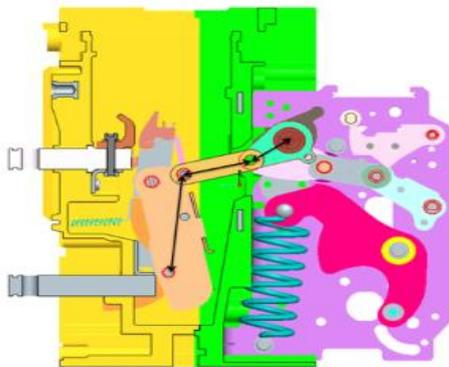
Figure 5: The existing Contact carrier assembly
