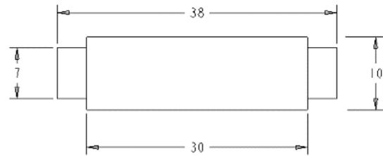
Figure 8: Delatching Pin dimensions
