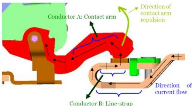
Figure 6: Reverse loop force at the contact
