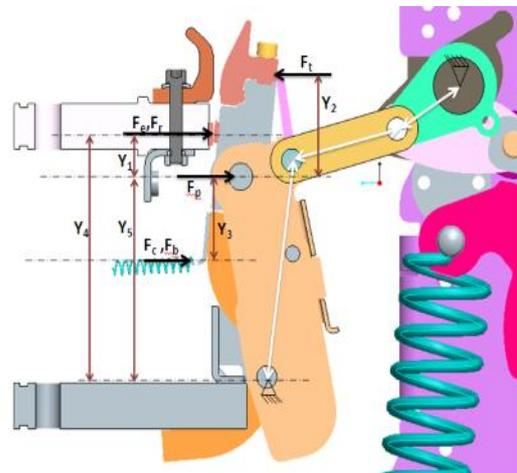
Figure 4: Forces acting on the contact system in ON position
