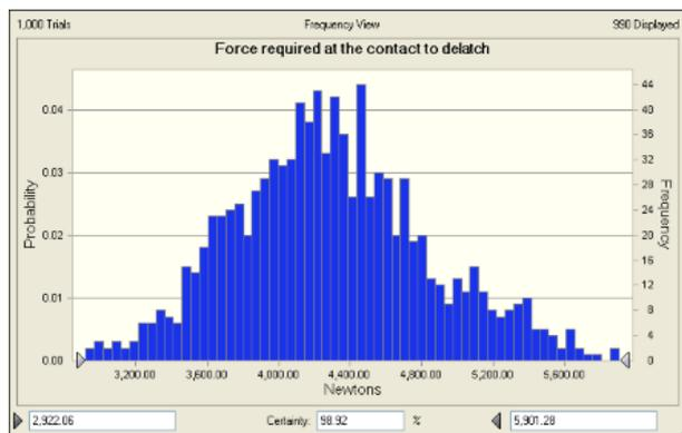
Figure 15: Forecast chart for the force required at the contact with Bushing
