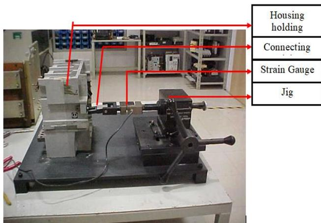
Figure 17: Test Setup for Prototype Testing
