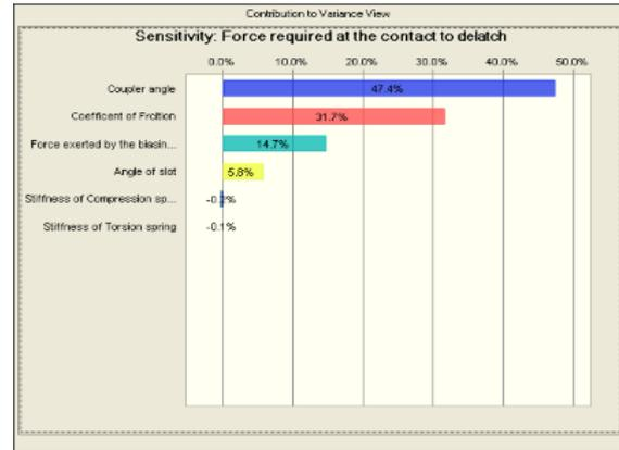
Figure 16: Sensitivity chart showing the contribution of each parameter with bushing
