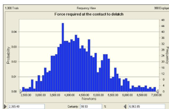
Figure 13: Forecast chart for the force required at the contact
