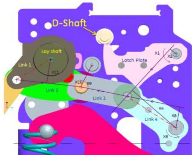
Figure 11: Transfer function to find torque required on Layshaft to rest
