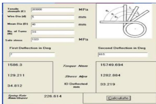
Figure 12: Torsion Spring Design tool
