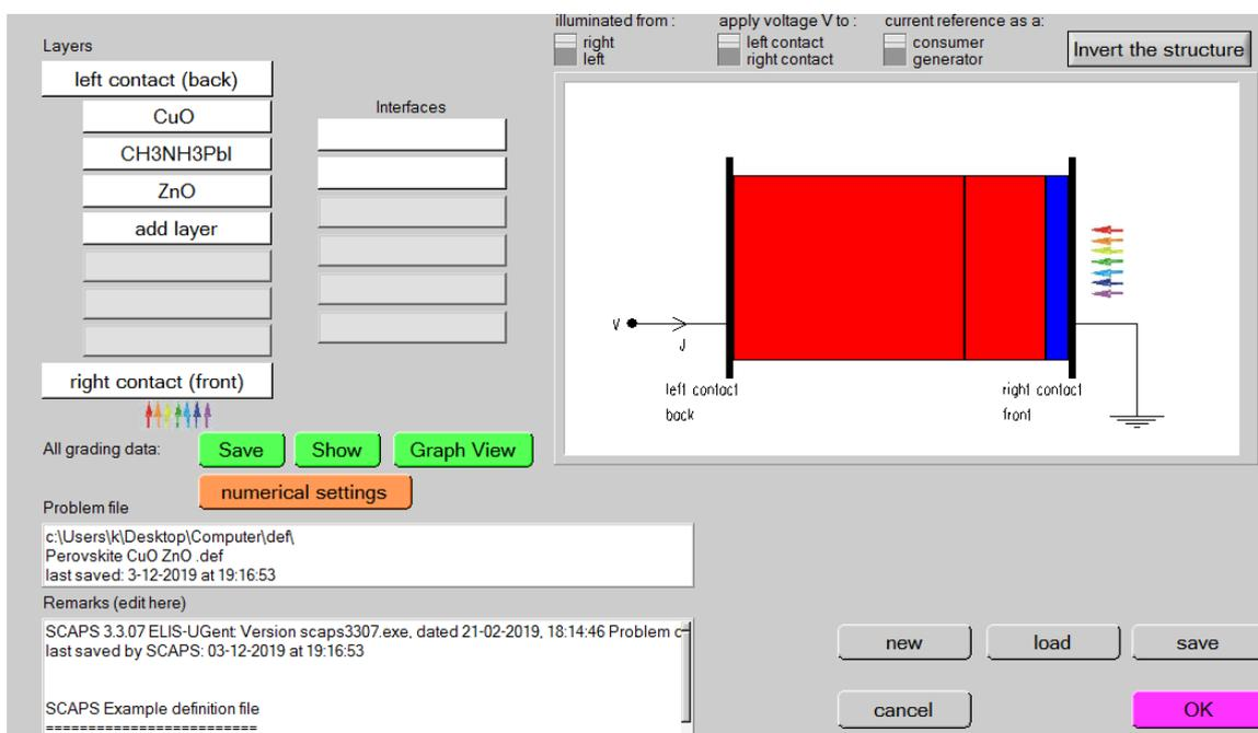
Fig. 4. SCAPS panel showing the CuO/CH3NH3PbI /ZnO hetrojunction solar cells definition
