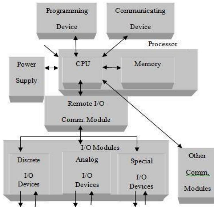
**Fig. 1: PLC architecture**
