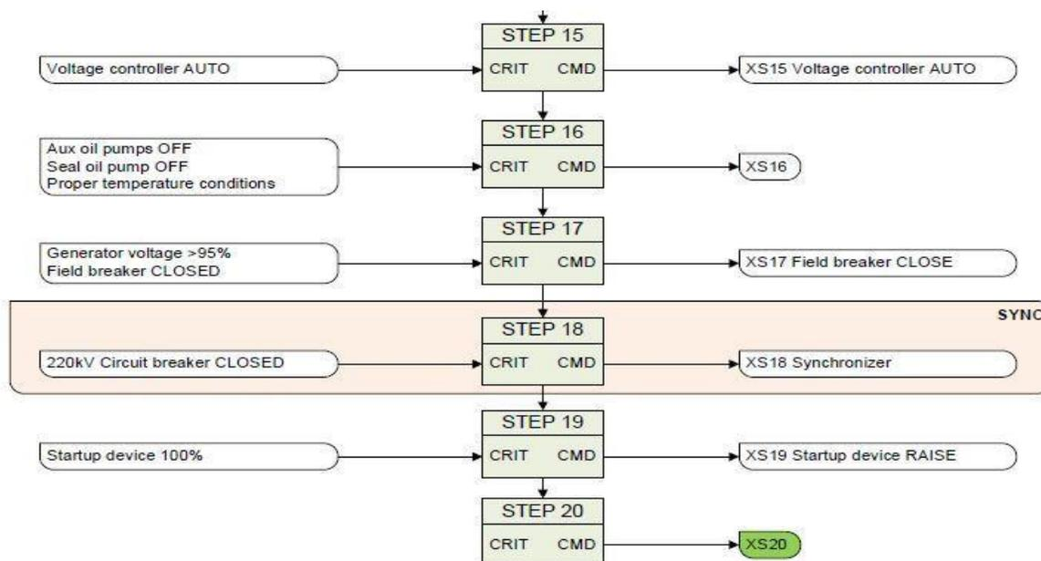
Fig 11: Start-up Sequence Logic
