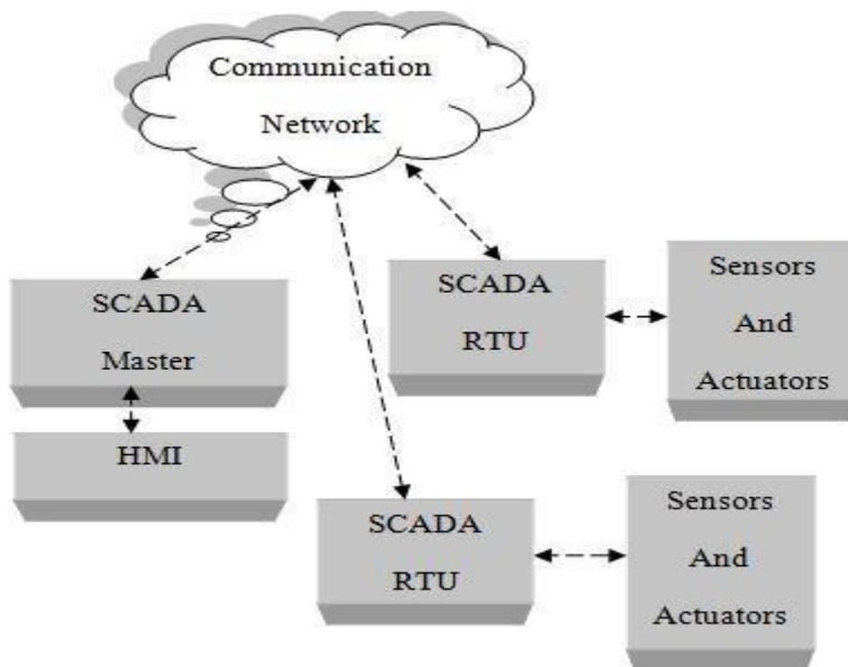
**Fig. 4: SCADA architecture**
