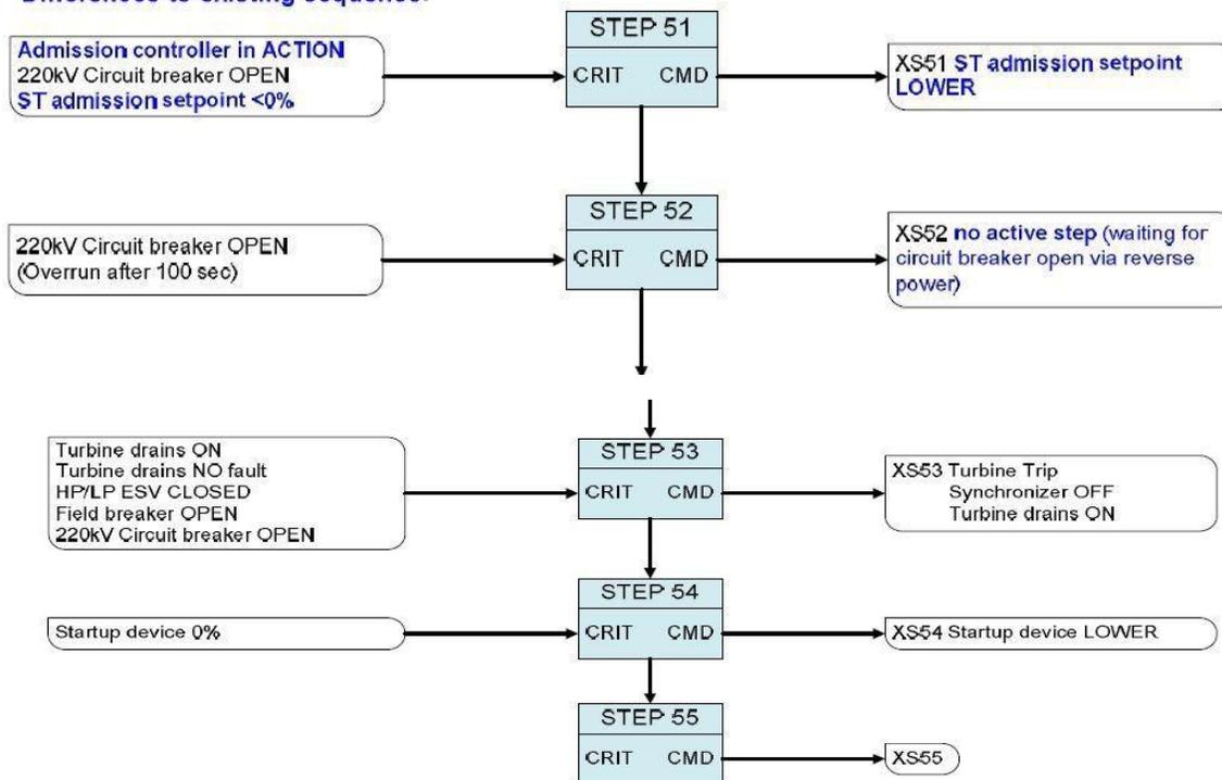
Fig 12: Shut Down Sequence Logic
