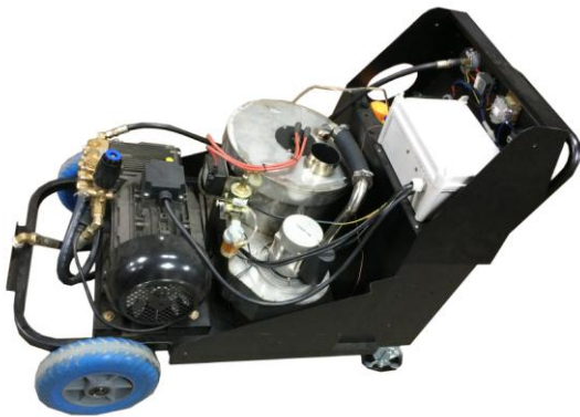
Figure 2. The Washing System that Sprays High Temperature High Pressure Hot Water
