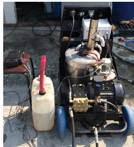
Figure 3. Performance Experimental System for the Washing System that Sprays High Temperature High Pressure Hot Water
