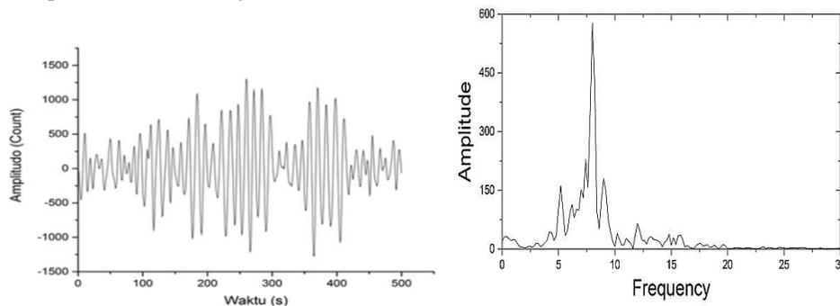
Figure 3. Examples of the waveform and spectral of a seismic event at Cangar on May 30, 2018 at 01:25:00 Western Indonesian Time.
