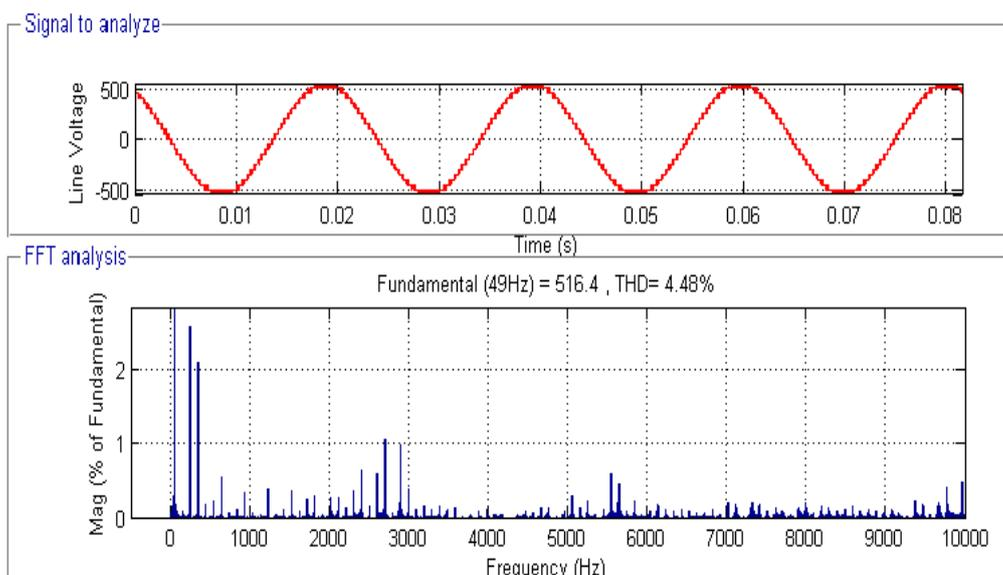
Fig.10: 23-level Output Voltage Waveform and %THD for AA-5.
