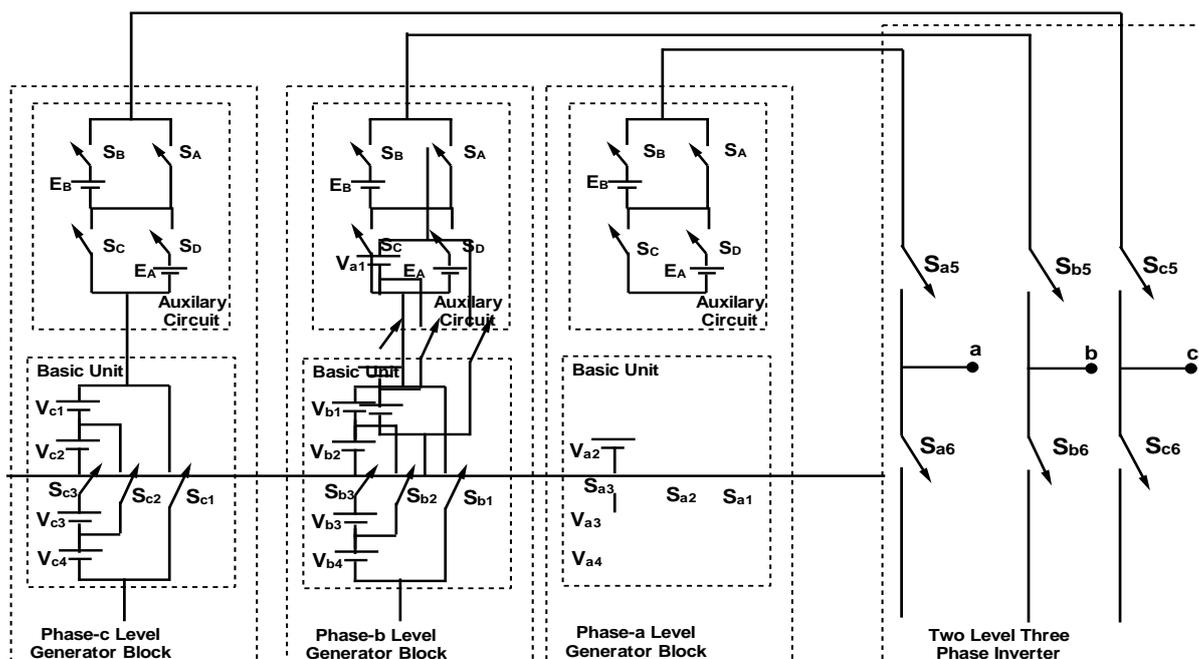
Fig.3:Proposedthree phase multi-level inverter topology.
