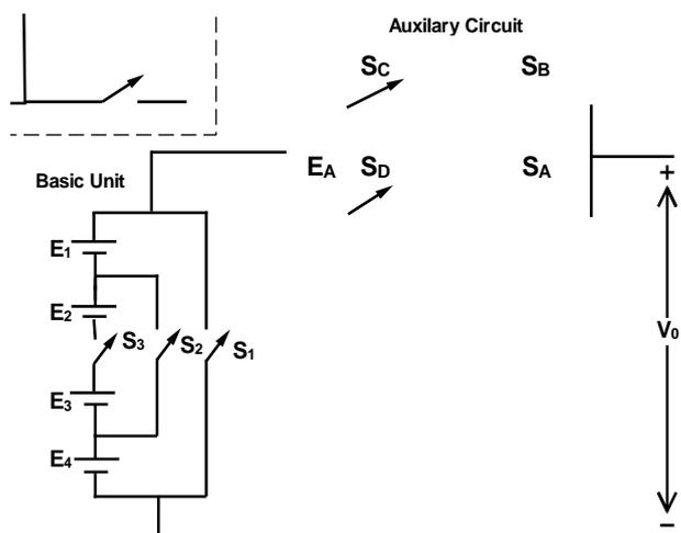
Fig..2: Level generator block for each phase
