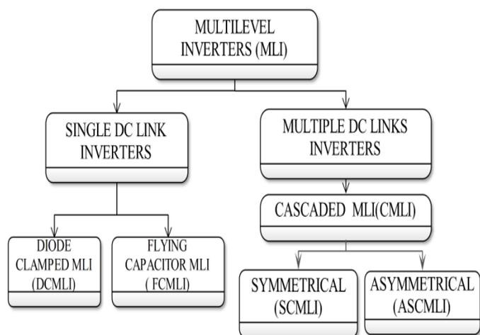
Fig.1: Types of Multi-level inverters
