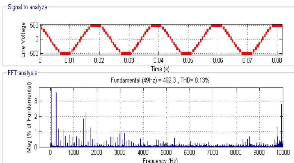
Fig.5: 13-level Output Voltage Waveform and %THD for SA
