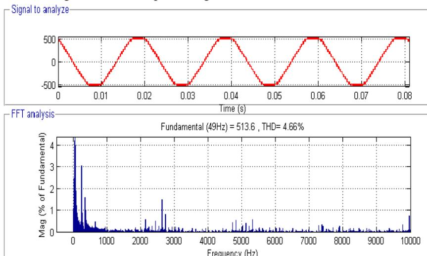
Fig.9: 21-level Output Voltage Waveform and %THD for AA-4.
