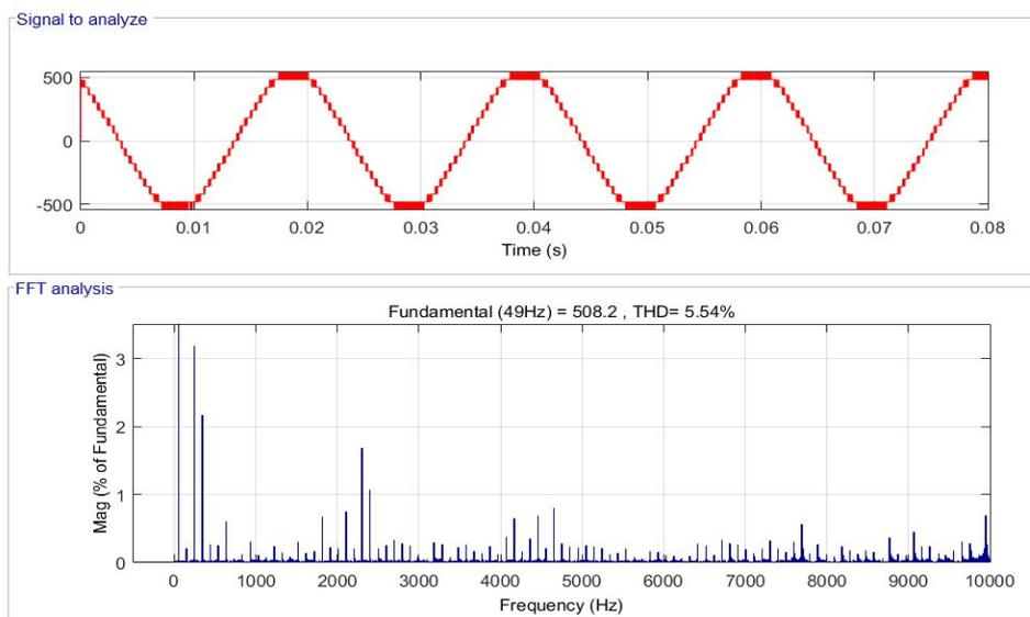
Fig.8: 19-level Output Voltage Waveform and %THD for AA-3.
