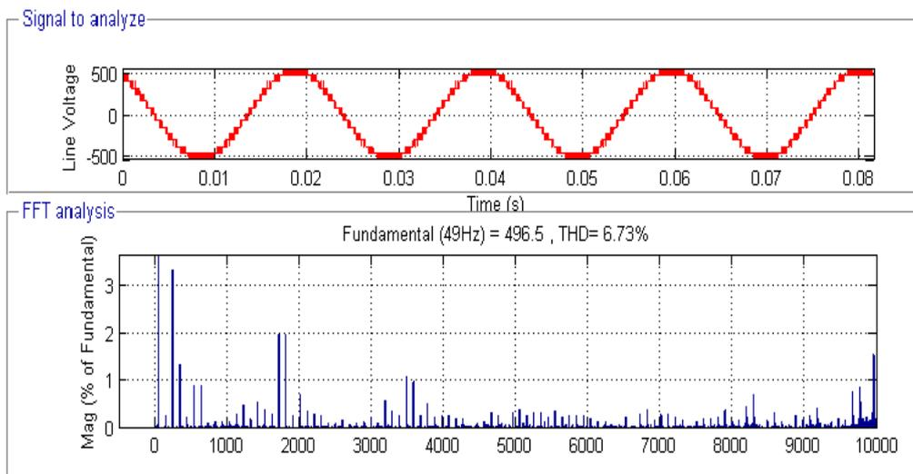
Fig.6: 15-level Output Voltage Waveform and %THD for AA-1.
