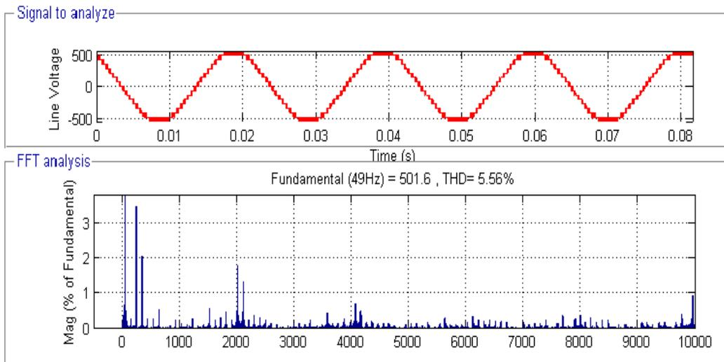
Fig.7: 17-level Output Voltage Waveform and %THD for AA-2.
