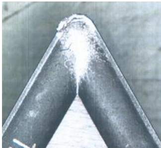
Figure 4 - Coated tool machined under dry environment
