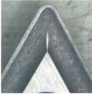
Figure 3 - Coated tool machined under wet environment
