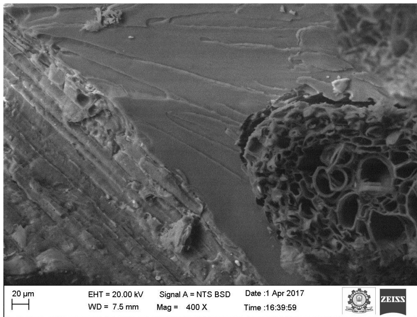
Fig. 6. Fractography image of 25mm, 35Wt.% of caryotafiber reinforced composites
