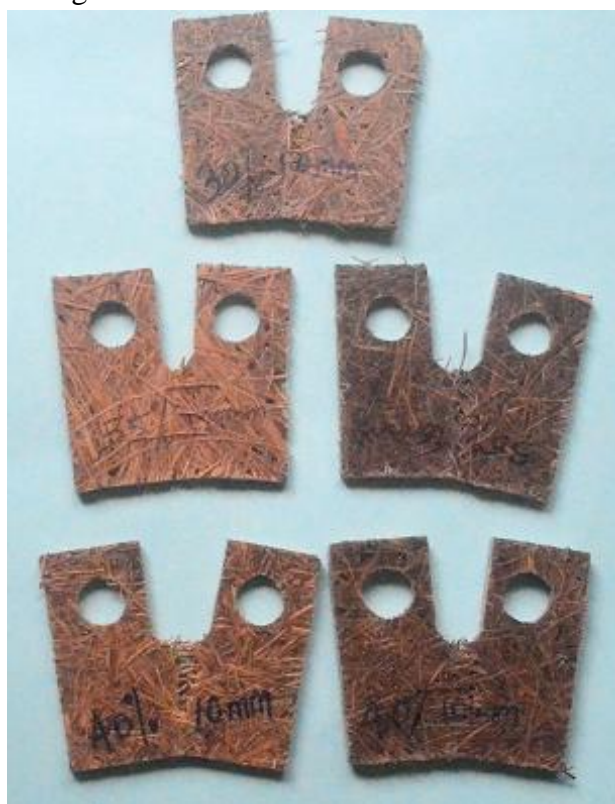
Fig.1. 40Wt% of 10mm, 25mm, 50mm, 100mm and 125mm length of fractured specimen
