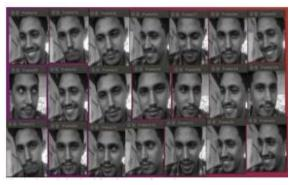
This image is the recognition results. This image depicts the various faces of one person that are recognized by the camera. Several angles of faces that are recognized by the camera are shown in this image. The attendance is marked even if anyone these faces are recognized by the camera.
