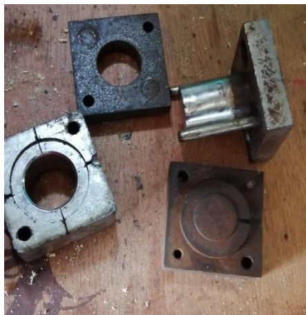
Fig (vi) Construction of the die
