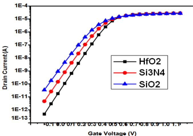
**Figure 11 Effect of Gate Oxide material variation at log Scale**
