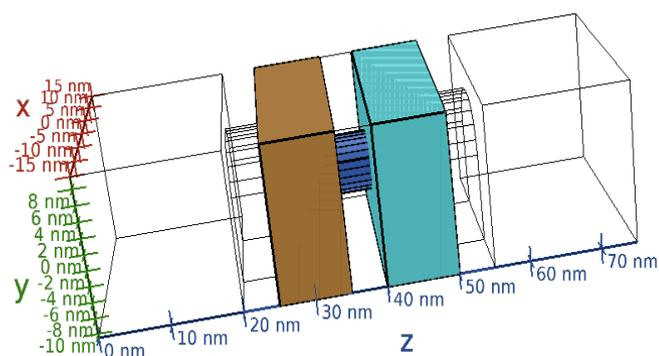
**Figure 7 Device showing Drain/Source Spacer region**
