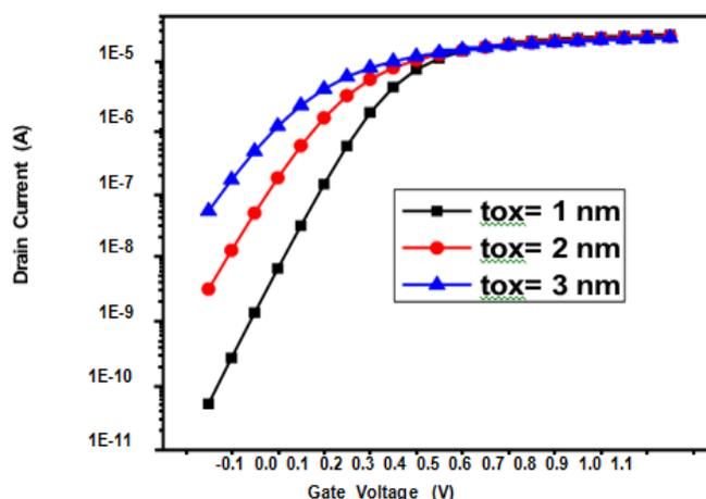
**Figure 9 Effect of Gate Oxide thickness variation at linear Scale**
