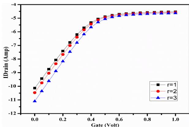
**Figure 6 Influence of channel radius on Drain current at log scale.**
