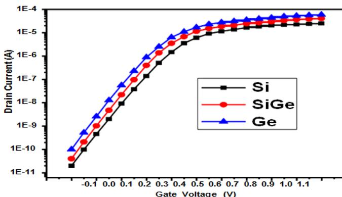
**Figure 18 Influence of different channel materials on Drain current at log scale**
