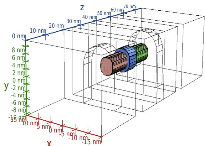
Figure 2 Nanowire Channel 3D Structure
