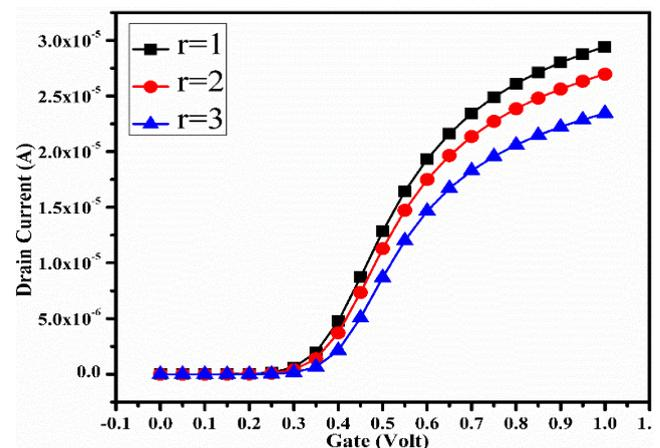
Figure 5 Influence of channel radius on Drain current at linear scale.
