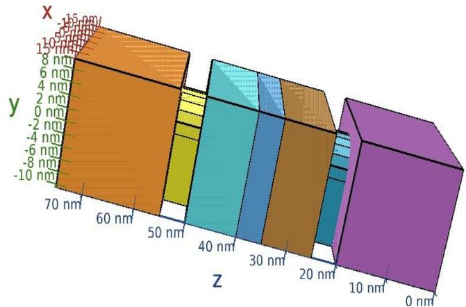
Figure 1 Complete 3D Structure of GAANWFET
