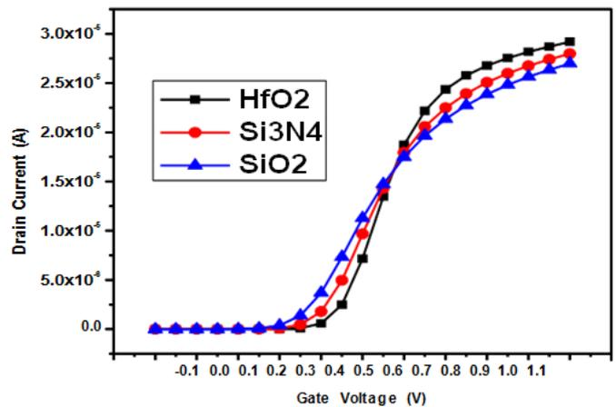
**Figure 12 Effect of Gate Oxide material variation at linear Scale.**
