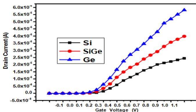
**Figure 17 Influence of different channel materials on Drain current at linear scale**
