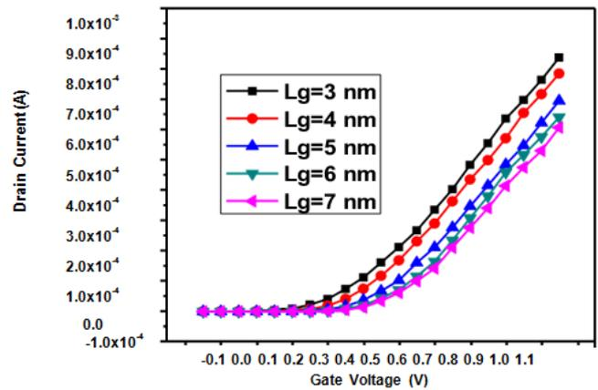
Figure 4 Id vs Vg Curve at Different Channel Length on Linear Scale.
