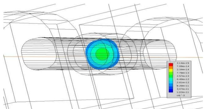
**Figure 13 Channel Electron Concentration 2D cutline profile**
