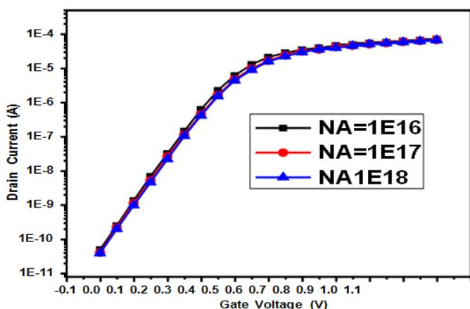
**Figure 15 Id-Vgs curve of Different Channel Doping Concentrations in log scale**
