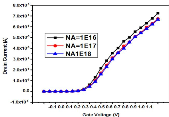
**Figure 16 Id-Vgs curve for different channel doping concentrations in linear scale**
