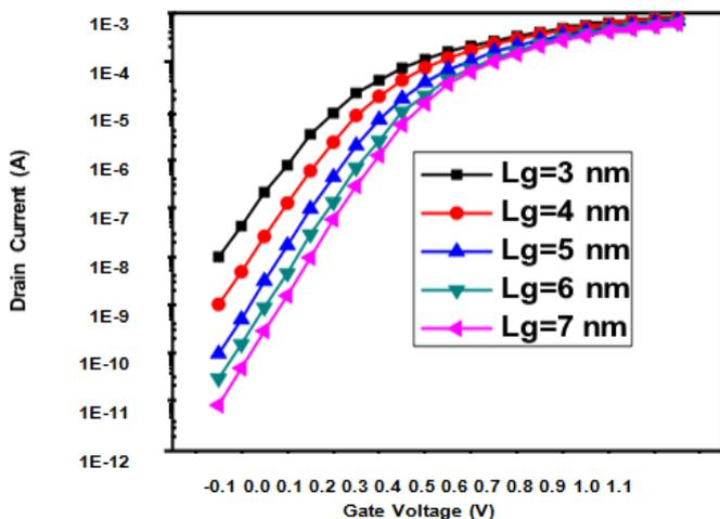
Figure 3 Id vs Vg Curve at Different Channel Length on Log Scale.
