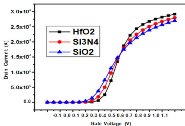
**Figure 8 Effects of different Spacer material on Drain current**
