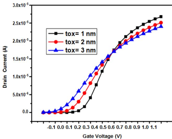
**Figure 10 Effect of Gate Oxide thickness variation at log Scale.**
