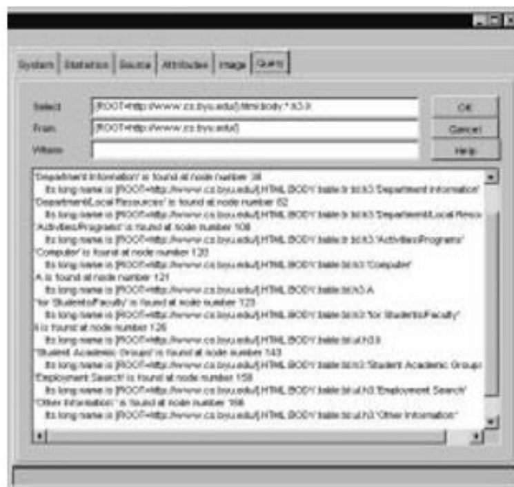
(b) Query Q_2 retrieves the data contents of headings of level 3 (h3)
