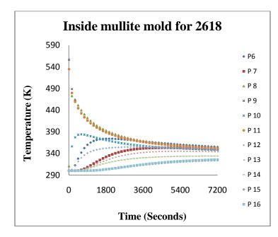
It observed in both systems, cooling curves convers but it is faster in case of the mullite mold.heating and cooling curves for mullite is more than sand this indicate addition heat transfer in mullite.
