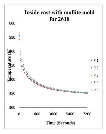
Uniformity of Slope of cooling curve for cast in sand mold shows that solidification taken place very slowly than to cast inside of the mullite mold.
