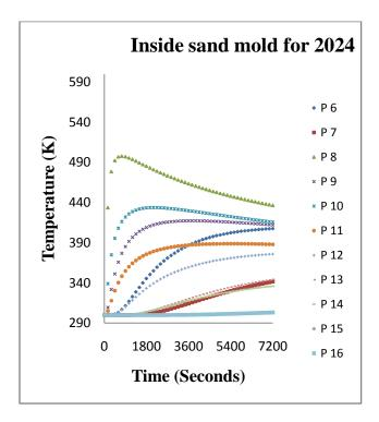
Due to suddentemperature decrement and increment showsan emphasizeddrop, with compare tothe sand mold.In heating curves the mullite molding are presented with points P14, P15, and P16 reason behind it thatthe location of these points are at a considerable distance from the casting.And other side, cooling curve inside the mullite mold does not exist.
