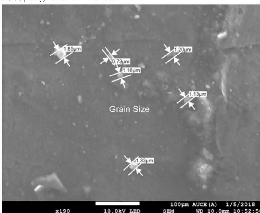
**Fig. 4 High UTS specimen of AA7075 with 9 wt% of marble dust SEM analysis**
