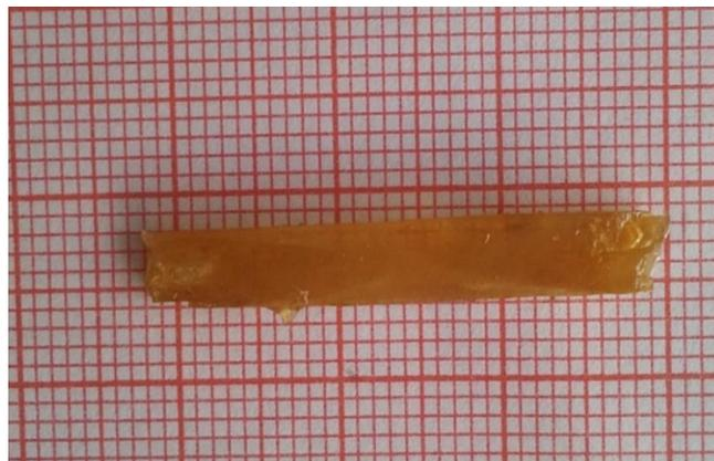
**Figure 1. As grown single crystal of 2APDM**
