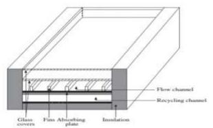
Figure 2: Schematic diagram of double pass internally finned solar air heater
