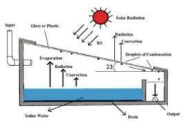
Fig.3. Working on the conventional single slope solar still
