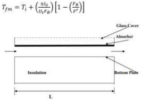
**Figure1: Conventional Solar Air Heater**
