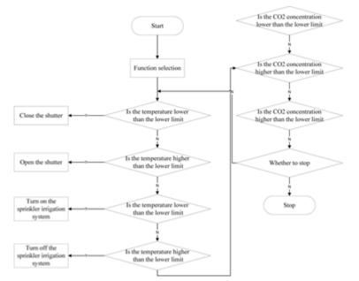
Figure 3. Flow chart of the automatic control system for greenhouses.
