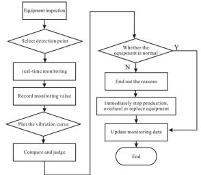
Figure 1. Flow chart of the inspection process of mechanical equipment.
