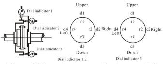
**Figure 4.** Schematic diagram of setting up a dial indicator with three-meter method and a diagram of the calibration data record.
