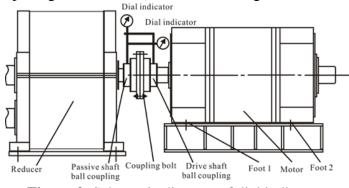
Figure 2. Schematic diagram of dial indicator installation and fixing methods.
