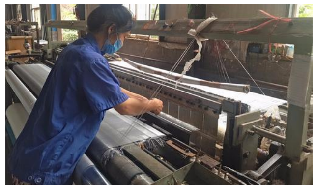
Figure 2. Alkali - resistant glass fiber made by hand.
