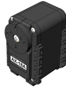
**Fig. 3. Solidworks model of the Digital servo**
