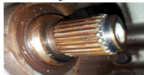
Fig 29: Actual spline condition after test
