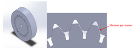
Fig.2. Involute spline coupling with maximum gap clearance.
