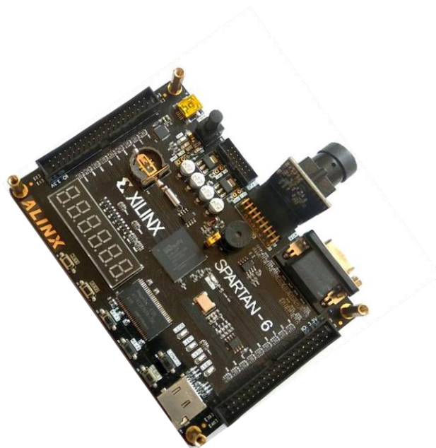
Figure 3: FPGA board with OV5640 Camera
