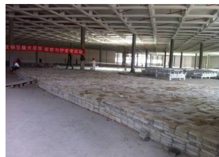
Fig.3 Local overload field test of an industrial factory building
