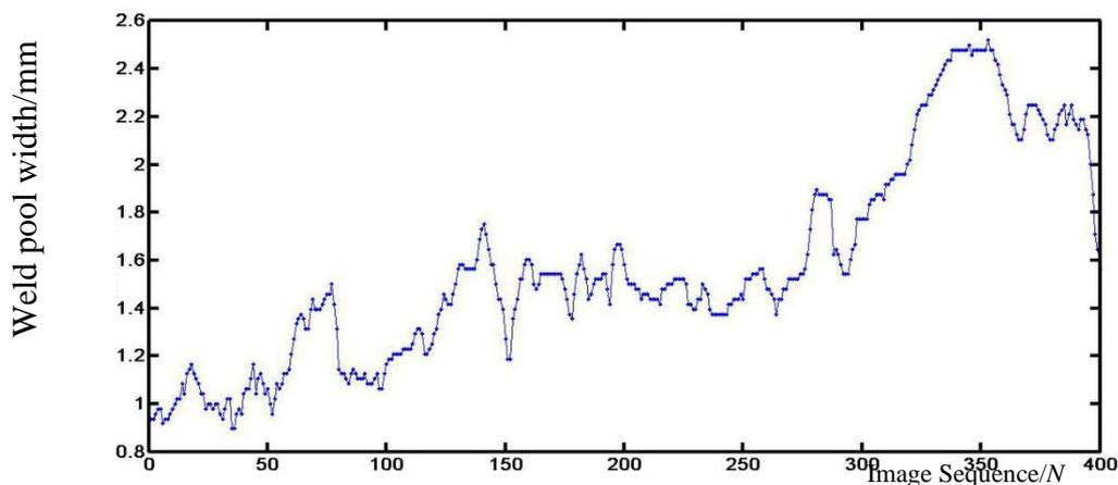
Fig.7. Weld Pool Width at the Back of Weld Seam
