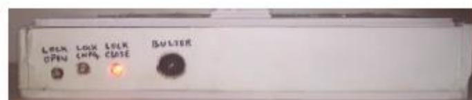
Fig. 11 Buzzer in status LED's for altering during times of unauthorized access
