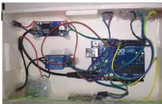
Fig. 12 Android based security system and its internal circuitry
