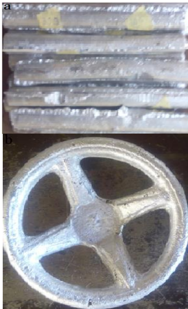
Figure 4: (a) Al-Mg-Cr alloy cylindrical rods cast and (b) Hand wheel cast from Al-Mg-Cr alloy
