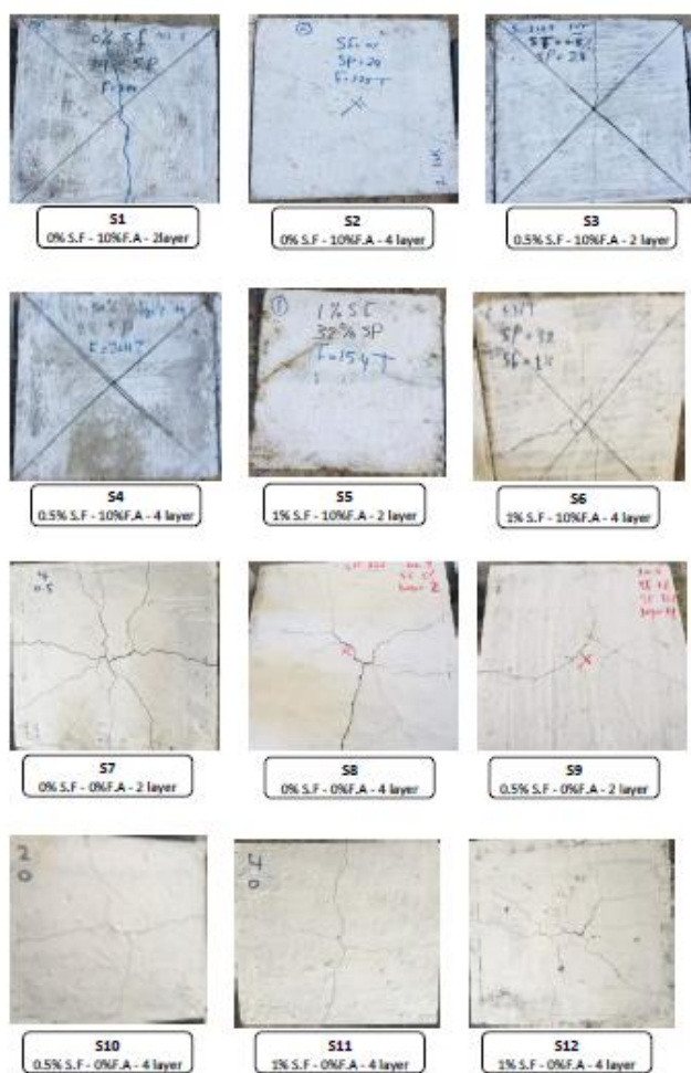
Figure (6) Failure modes of the tested slabs
