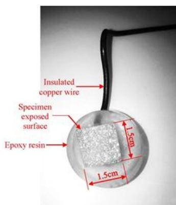
**Figure 1.** WE embedded in epoxy with exposed area of 2.25cm<sup>2</sup>
